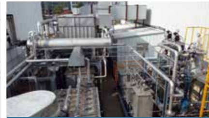
Recovery of organic waste gas in soft package industry Carbon fiber adsorption process
