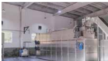
Surface treatment sludge drying project Daily processing capacity:8T
